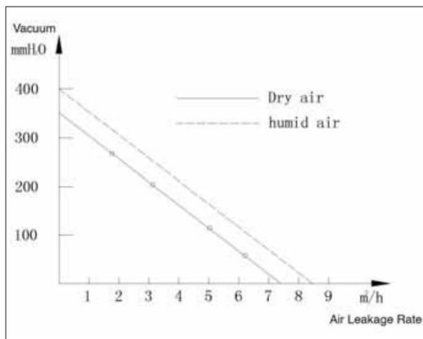
Figure 1: Air leakage rate at the beginning of refrigeration and vacuum formation (ambient temperature +38°C, setpoint -20°C)
