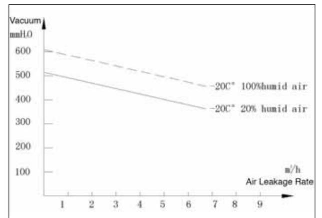
Figure 2: The relation between vacuum and air leakage rate when the reefer unit is stopped
