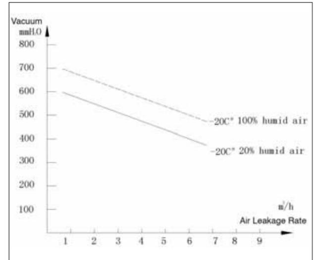
Figure 3: The relation between vacuum and air leakage rate when the reefer unit is running
