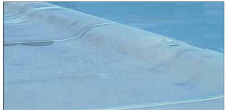
*Collapse of roof panel as a result of a vacuum forming inside the container*
